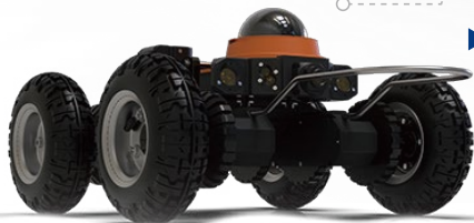
▶ wheel drive module for larger diameter pipes
